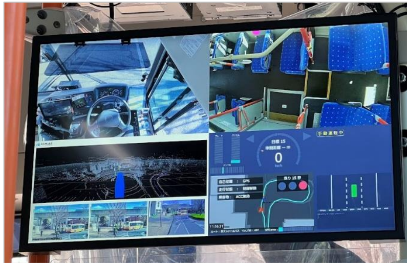
Figure 2 - Image of a display installed in the automated driving bus
