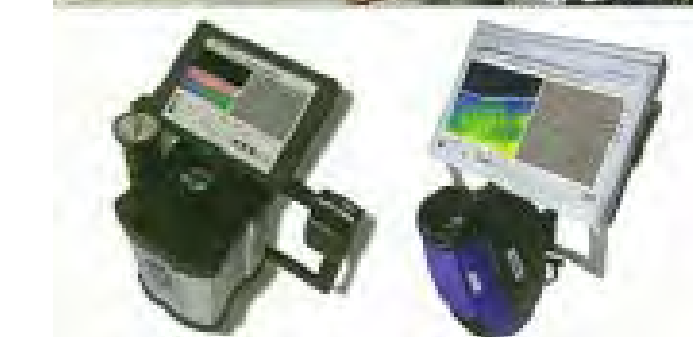
Bridge inspection using Infrared Camera System
