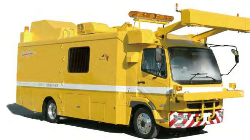
High-Speed Road Surface Measuring Vehicle (Road Tiger)
