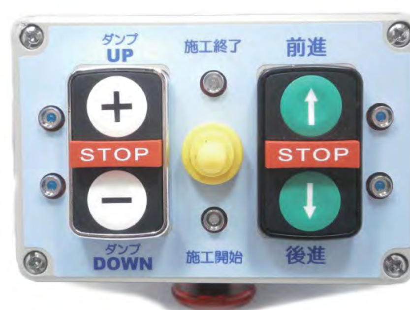
Hard-wired switch box
